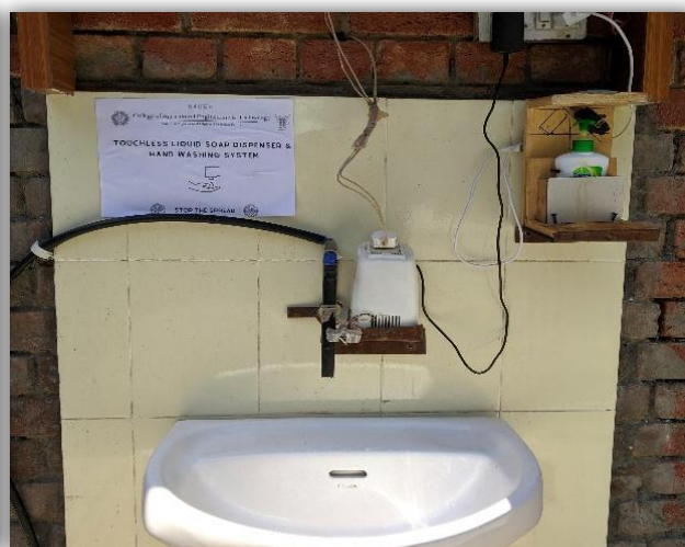
Contactless liquid soap dispenser cum hand washing system invented by students of COAE
